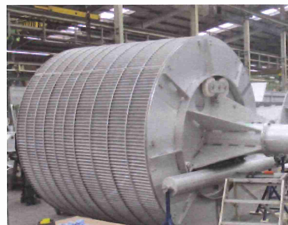
HUBER Perforated Plate Screen ROTAMAT® STAR, 2600 mm diameter, 1 mm perforation
