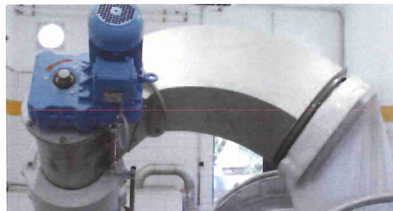
Individually adapted installation with lateral screenings discharge directly into a container
