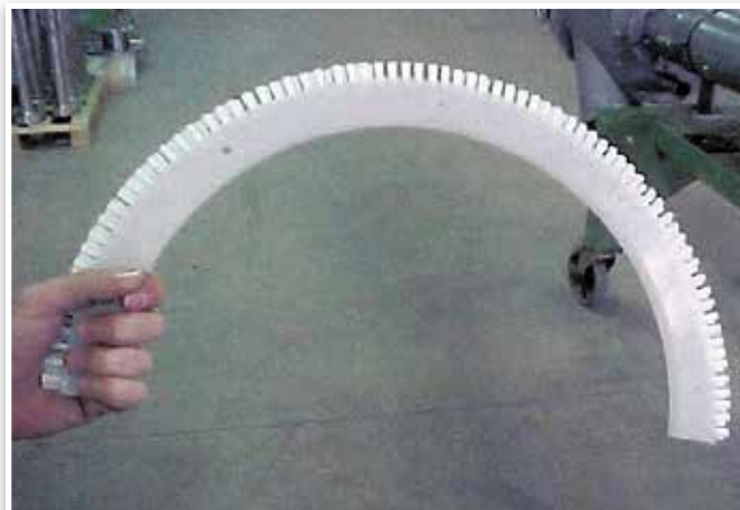
Easily Replaceable "Bolt On" Brushes.
